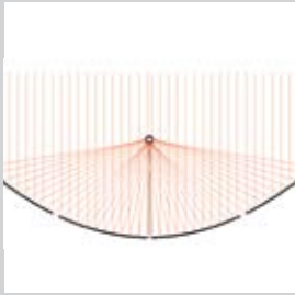
Ray tracing of parabolic trough mirrors
