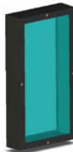
Drawing no.5 Polyurethane frame moulded onto the windshield
