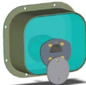
Drawing no.2 Carbon steel frame with gunport in the window
