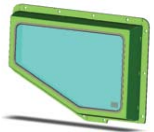
Drawing no.3 Combination of armor and carbon steel frame
